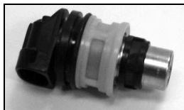
Bottom-Fed Fuel Injector
