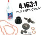
Transfer case gear reduction kit reduces Transfer Case gear ratio from a stock ratio of 2.268 to 4.163. Hi-range reduction of 12.2%. This will allow the use of tires up to 30" in diameter without making axle gear changes. Comes complete ready to install in your stock transfer case housing without modification. Kit includes gaskets, oil & installation instructions 86-95 Samurai / SJ413 Part #SS5025
