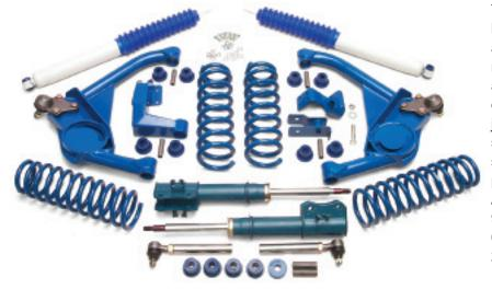
CALMINI does it right! We offer a system that truly improves every aspect of the vehicles off-road ability. Replacement control arms that provide lift, increased ground clearance, and most importantly maintain stock track width, is the only way to go. Longer control arms also increase wheel travel. The spring rates we designed offer greater load carrying capacity. Also, it's fully bolt-on. This is a suspension system, not just a lift kit.
