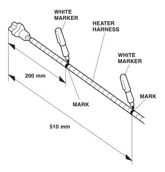
Plug the heater harness connector into the engine block heater. Route the heater harness along the vehicle harness and secure it to the vehicle harness with one wire tie at the white mark.
