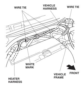
11. Continue routing the heater harness alongside the vehicle harness, and secure the heater harness to the vehicle harness with three wire ties.
