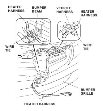
Secure the heater harness to the bumper grille with one wire tie.
