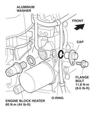
7. Insert the O-ring onto the cap, and install the cap into the hole of the engine with the flange bolt. Torque the flange bolt to 11.8 N·m (8.6 lb-ft).
