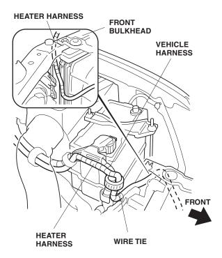
13. Continue routing the heater harness along the vehicle harness through the front bulkhead to the center of the bumper grille. Secure the heater harness to the vehicle harness and bumper beam with two wire ties.
