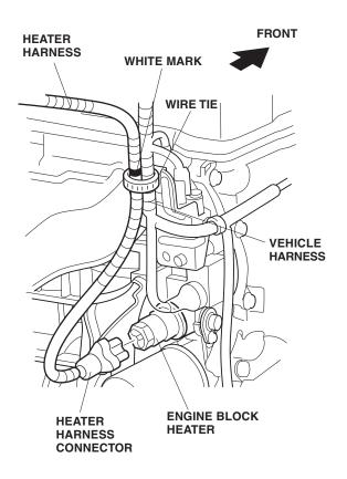
10. Route the heater harness alongside the vehicle harness, and secure the heater harness to the vehicle harness and frame with four wire ties.
