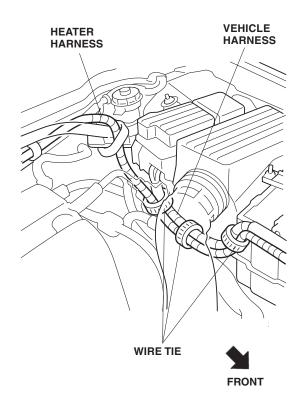
12. Continue routing the heater harness along the vehicle harness through the front bulkhead to the right side of the radiator. Secure the heater harness to the vehicle harness with one wire tie positioned on the inside of the front bulkhead.
